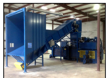
'Walking Floor' Truck Unloading and Baling System
